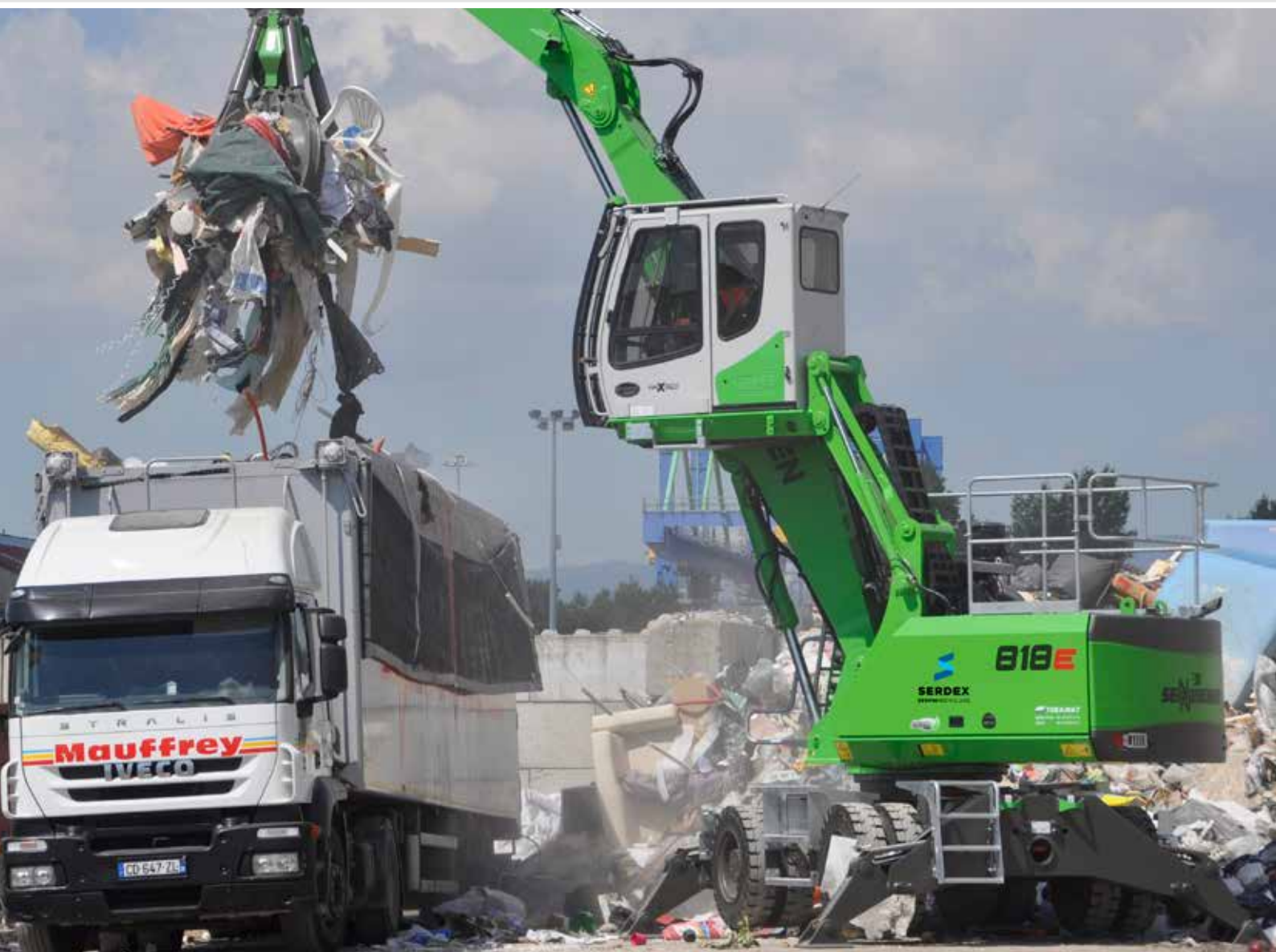
Schrottschere statt Stiel Scrap shear instead of stick
