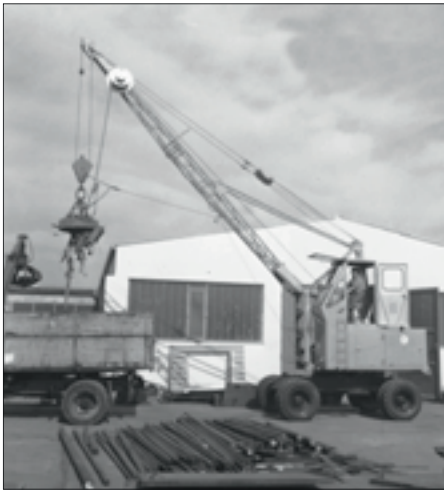
1962: rope-driven S833 with elevated operator cab
