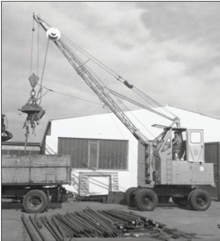
1962: Rope-driven S833 with elevated operator cab
